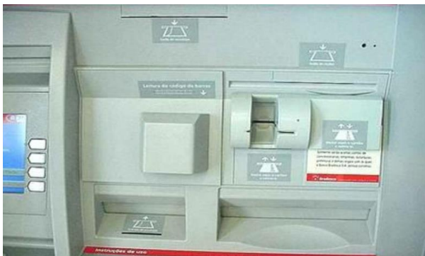
Installed in front of the existing bank card slot. PIN reading camera being installed.
