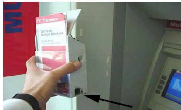
Installed in front of the existing bank card slot. PIN reading camera being installed.
